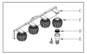
Step.4: Position Glass(F) onto the socket of fixture body(C), then secure with socket ring(D) with Glass(F) onto  $Fixture\ body(C)$  by using spanner(E).
