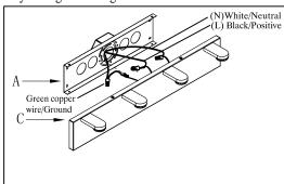
Step.2: Wire fixture to wires in outlet box. Green copper wire is for ground. And carefully position all wires inside the outlet box.
