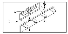
Step.3: Place the fixture body(B) against mounting bracket, Align the two holes of the mounting bracket and fixture body, then tighten the screws(C).
