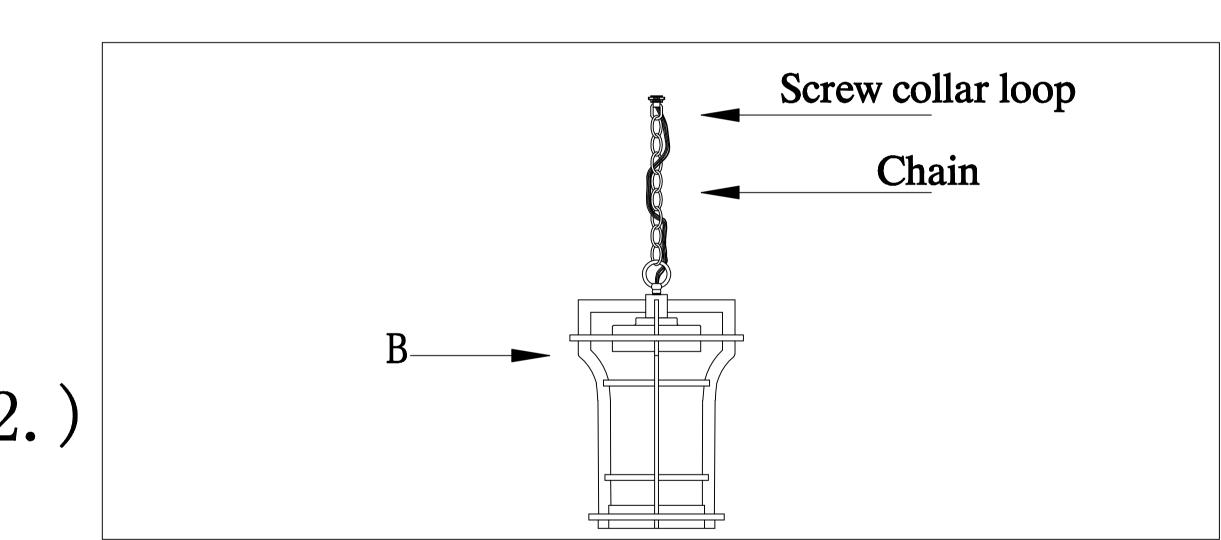
Step.2: Install chain to fixture(B), install screw collar loop to chain. Attach appropriate amount of chain to loop to achieve desired mounting height. Thread wire through every 3rd loop of chain.
