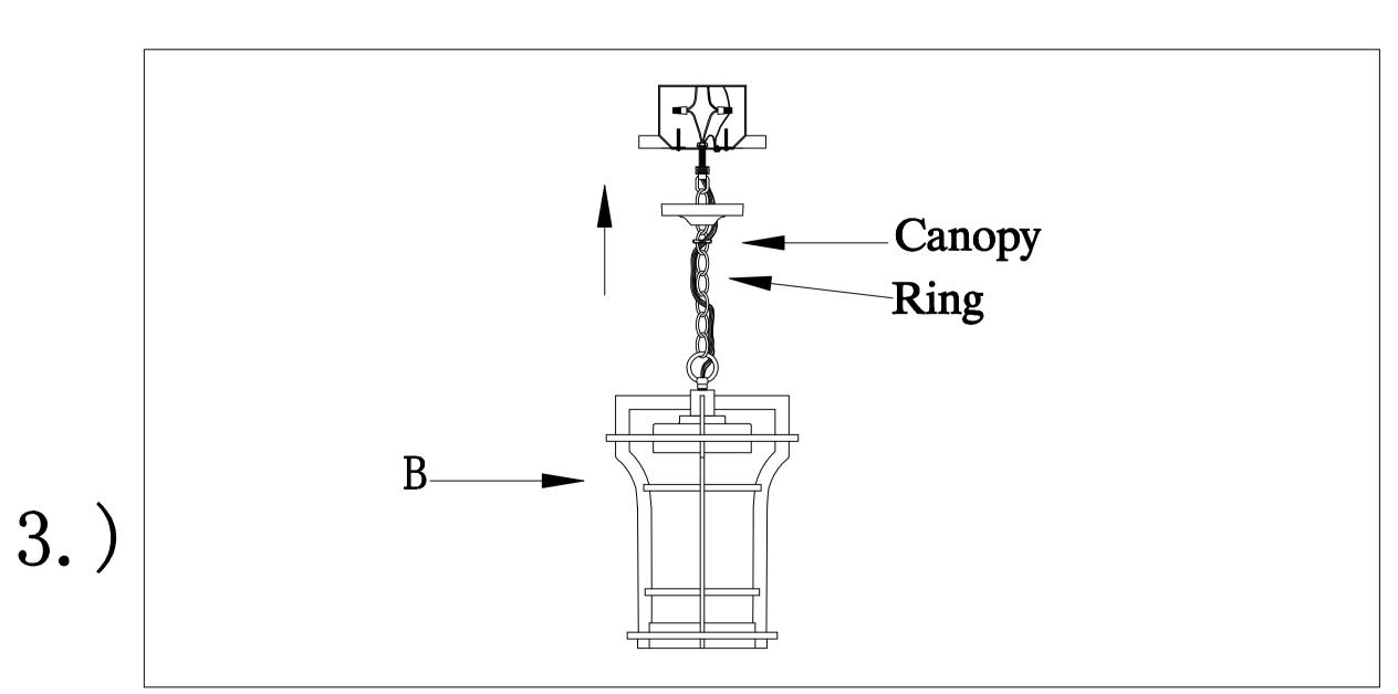
Step.3: Remove ring from loop and slide down chain. Place canopy onto chain and let slide to top of fixture. Install screw collar loop to bracket. Pull canopy through screw ring up chain to ceiling and tighten securely.
