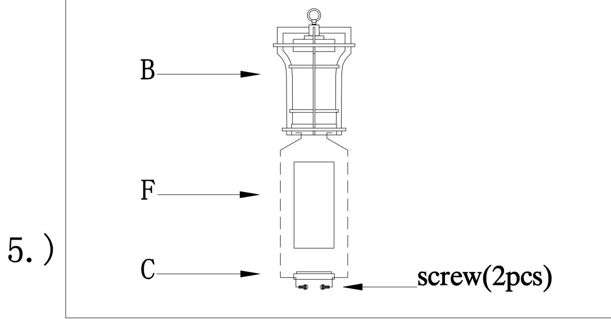
Step.5:Install the outside glass(F) to fixture; install the bottom ring(C) to fixture(B) with two screws.
