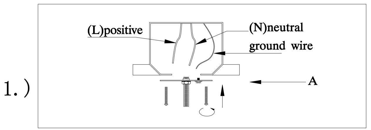
Step.1: Remove mounting bracket(A) from fixture and install to electrical box.
