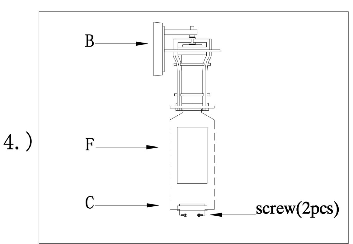
Step.4:Install the outside glass(F) to fixture; install the bottom ring(C) to fixture(B) with two screws.
