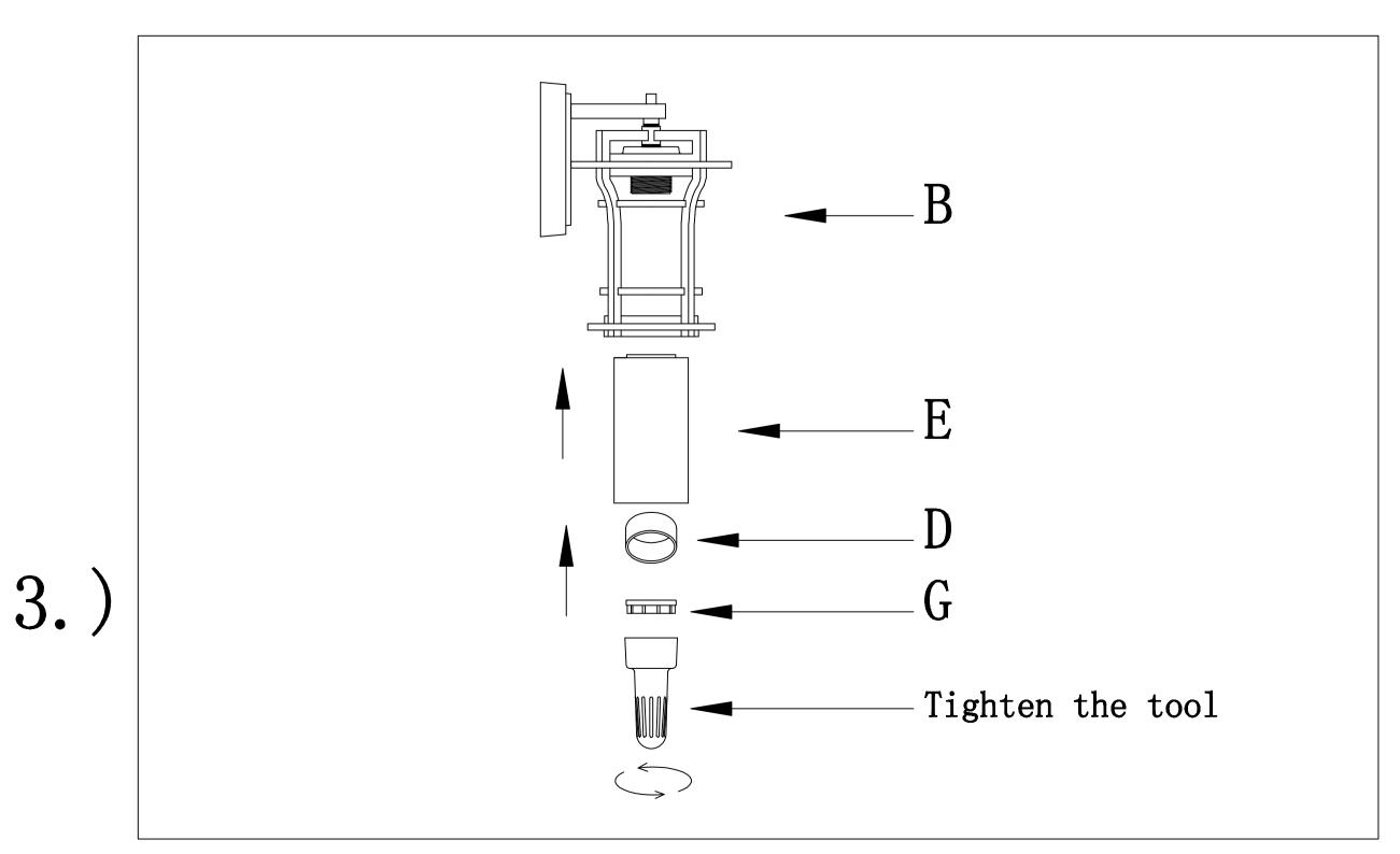
Step.3:Install the inside glass(E) to fixture(B); install the casing(D) and the screw ring(G) to fixture using tighten the tool.
