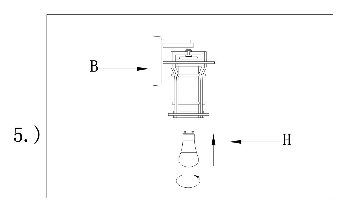
Step.5: Install GU24 LED bulb(H)
