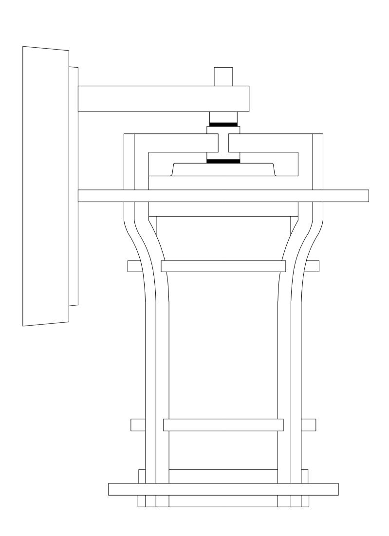
To prevent water intrusion, caulk around back-plate where fixture meets the wall using outdoor silicone sealant. Leave a small gap at the bottom to allow moisture to exit.
