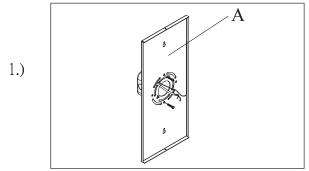
Step.1: Install Mounting bracket(A) to outlet box.
