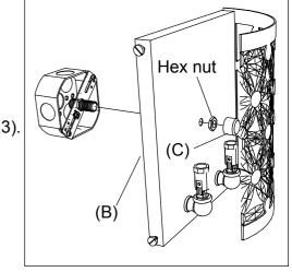
Step.3: Install body (B) to the outlet box and secure with hex nut and Decorative nut (C). Place the Candle Tube (E) and Cap (D) onto the socket, Install light bulb.
