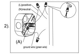
Step.2: Wire fixture to wires in outlet box. Silver & Copper wire is for Ground.
