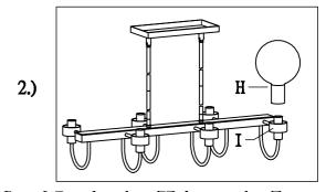
Step.2:Put the glass(H) into socket(I) one by one
