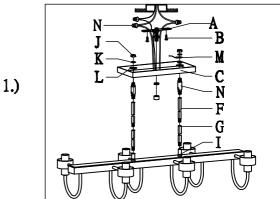
Step.1: Remove Crossbar from fixture and install to electrical box
