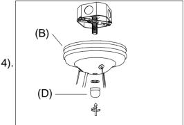
Step.4: Install body (C) to Mounting Strap (A) and tighten nut and ball nut (D) on the canopy to secure. Install crystal (E) on the arm. Insert bulb (F) in the socket.
