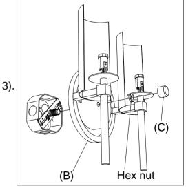
Step.3: Install body (B) to the outlet box and secure with hex nut and Decorative nut (C). Install finial (D) on the body. Place the Candle Tube (E) over the socket, Install light bulb.
