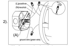
Step.2: Wire fixture to wires in outlet box. Copper wire is for Ground.
