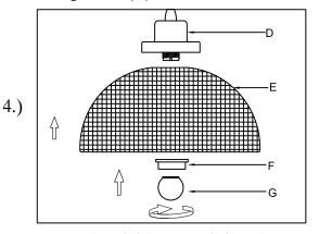
Step 4: Insert glass (E) into cup (D) and secure using Aluminum loop (F) provided, At last Screw (G) to the lamp holder.
