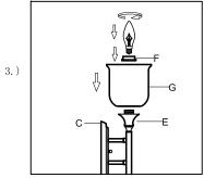
Step.3: Put the glass (G) with the covers (F) into the cup (E).Use Max 60W bulb.
