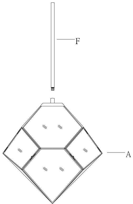
1. Run wire through stems and combine stem lengths to meet desired mounting height
