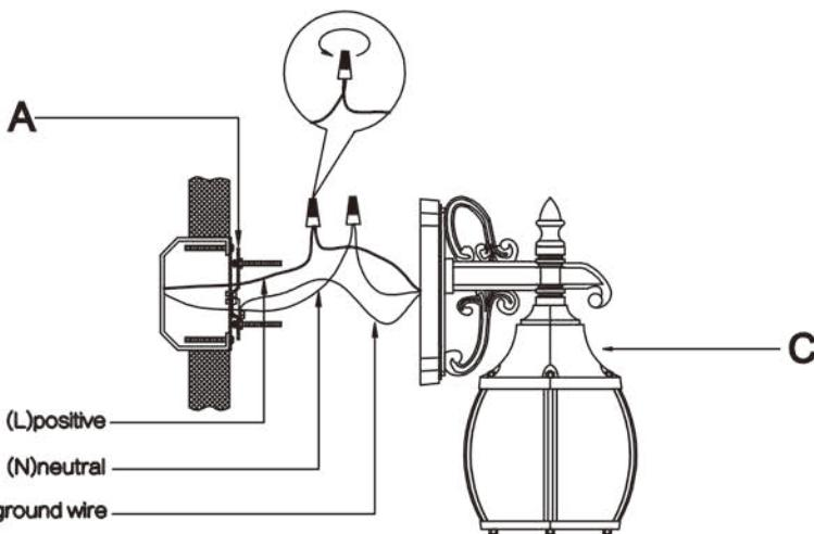
2. Caulk around backplate where fixture meets the wall leave a hole at the bottom to allow water to escape.
