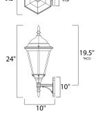
\*height from the center of outlet to the top of the fixture
