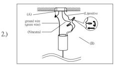
Step.2: Wire fixture to wires in outlet box. Install Green wire to Ground Screw.
