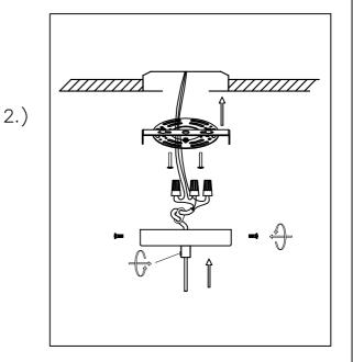
Step.2: Adjust wire length to desired mounting height, and tighten strain relief screw (D) to secure. Wire fixture to wires in outlet box. Green wire is for Ground. Install fixture to bracket and tighten screws (F) at the ends of the canopy (E) to secure.
