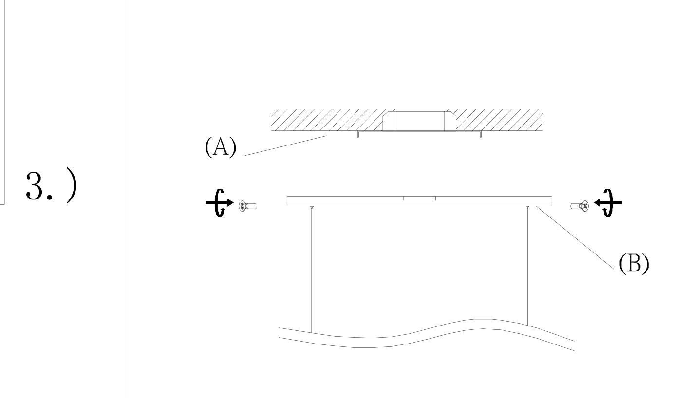
Step 3: Install Body (B) to Mounting Bracket (A) and tighten screws on the sides of the canopy to secure
