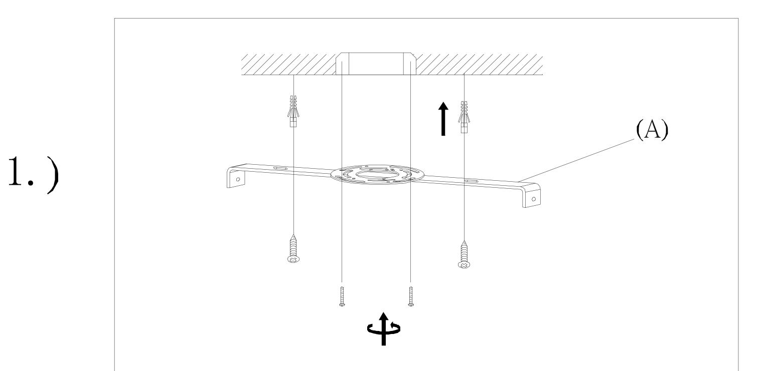
Step 1:Remove mounting bracket from fixture and install to electrical box Mark where screws at ends of bracket meet the ceiling. Remove mounting bracket from ceiling. Drill holes using 3/16"± drill bit where marked. Install mounting bracket to outlet box and attach anchors to secure bracket at
