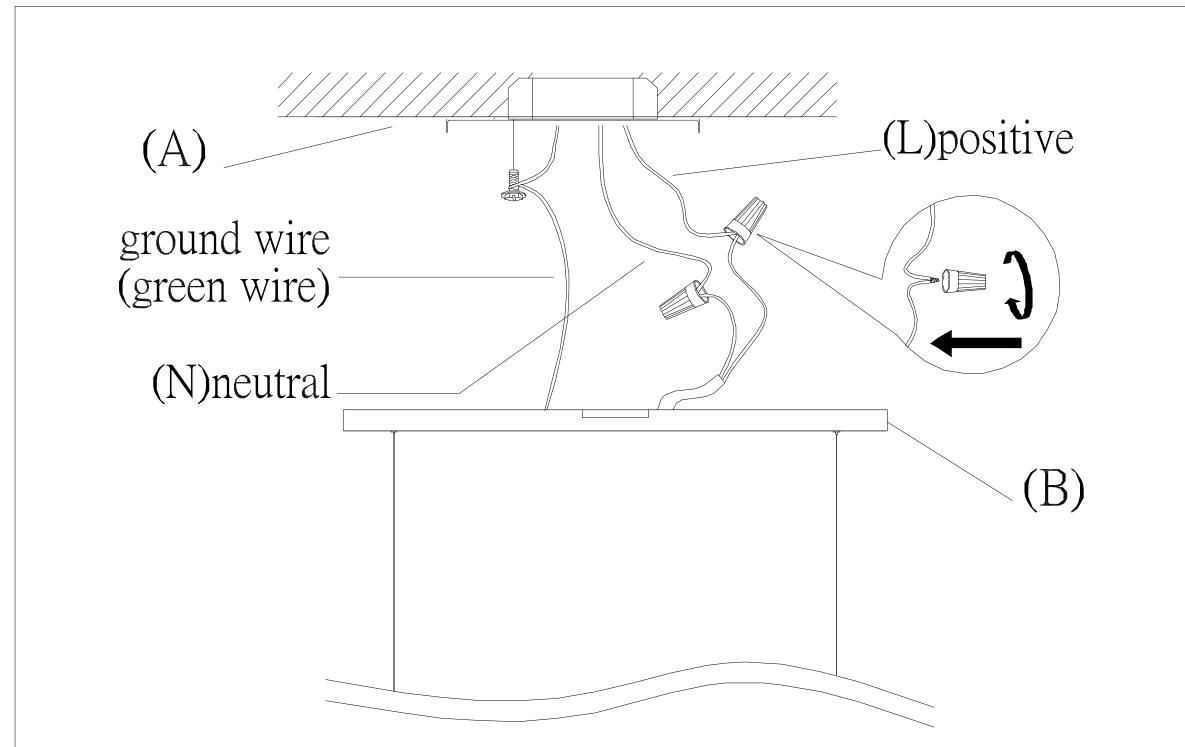
Step 2: Use push pins to adjust wires to desired mounting height. Wire fixture to wires in outlet box. See dual plastic wire instructions for more details. Install Green wire to Ground Screw.
