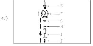
Step.4: Install Glass(F)/Cap(G) onto socket(E). Install socket ring(H) onto socket (E) by spanner (I). Then install G9 LED bulb (J) into socket(E).
