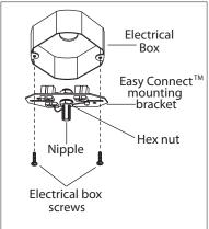
$\mathbb{1}_{\circ}$  Attach nipple to mounting bracket. Adjust so it will clear hole in back of fixture and then lock nipple in place with hex nut. Attach mounting bracket to electrical box with electrical box screws (not included).
